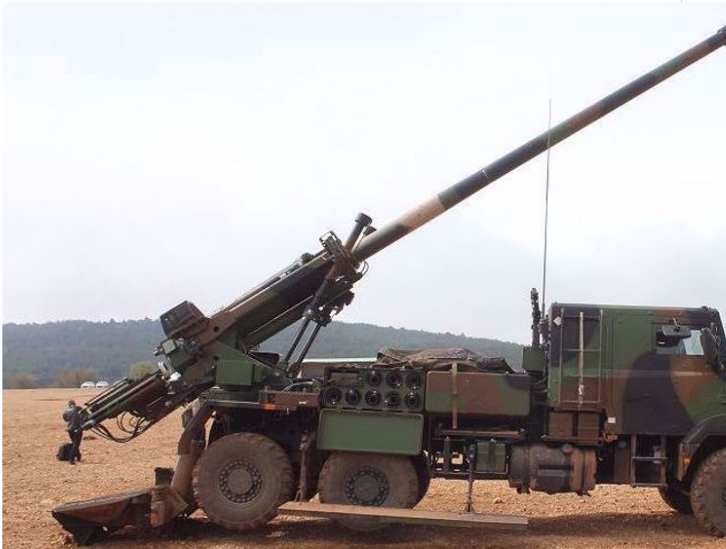
Photo shows a French Army CAESAR 155mm 6x6 wheeled self-propelled howitzer.
