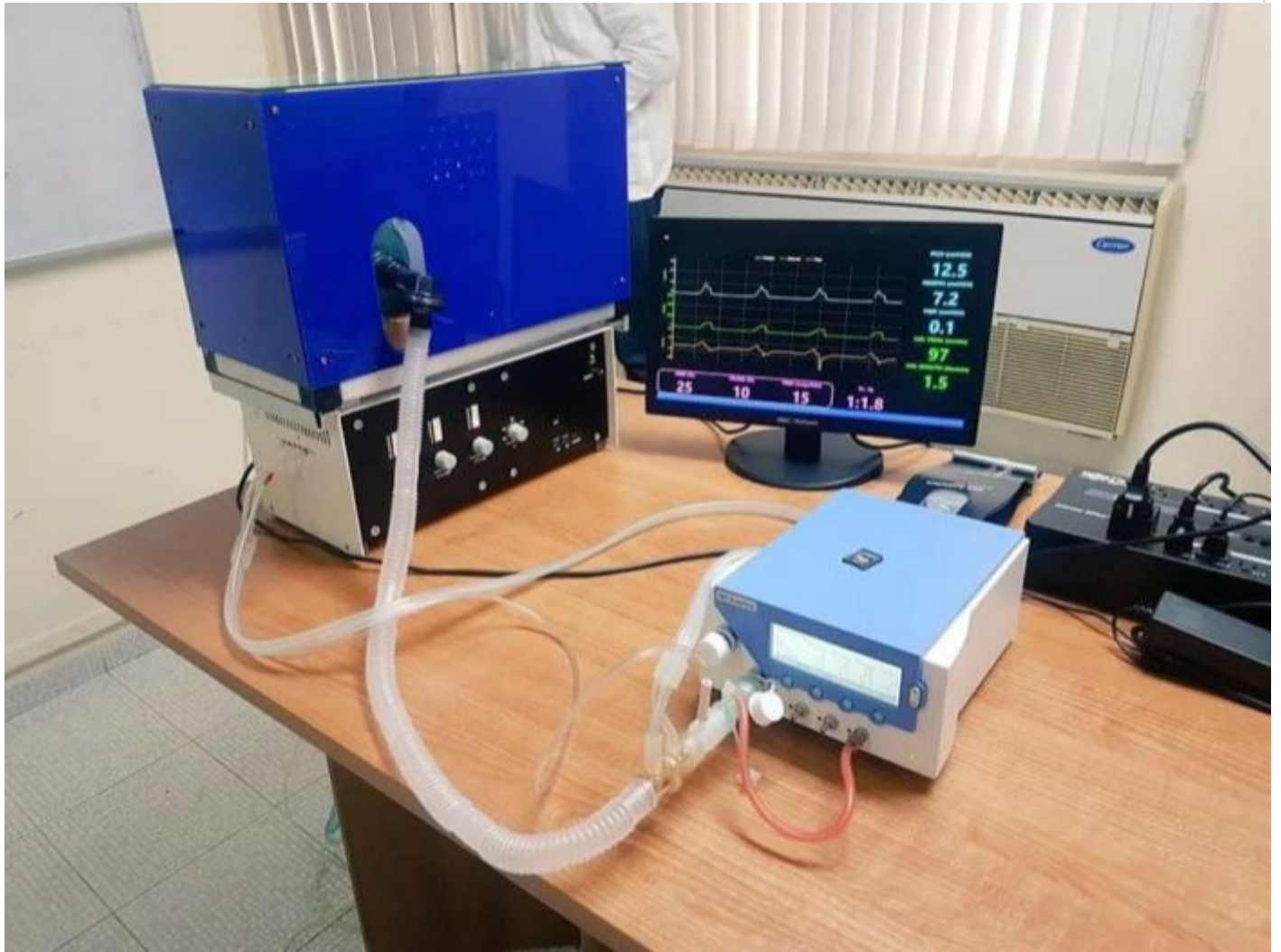
Cuban-made lung ventilator. GELECT photo
