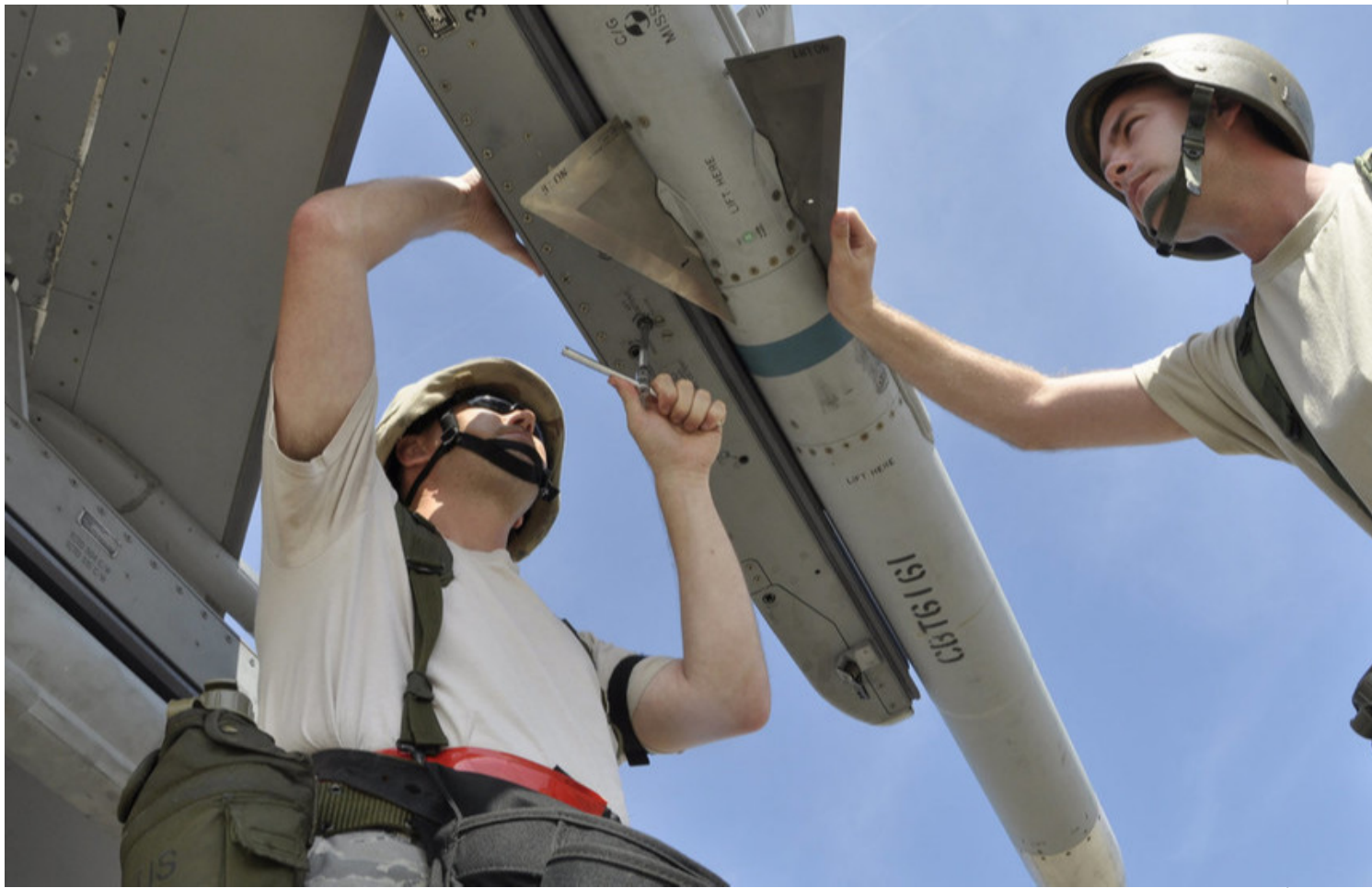
Members of the US Air Force engage the aft dampener on an AIM-120 AMRAAM missile © Flickr / US
